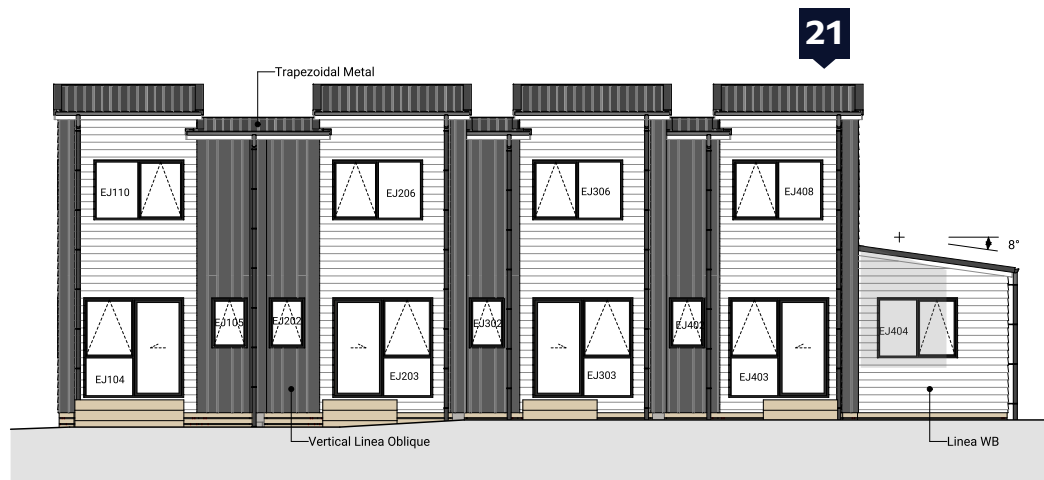
3 South West Elevation
